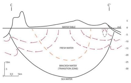
Figure 9.1: Cross section of East End Fresh Water Lens
