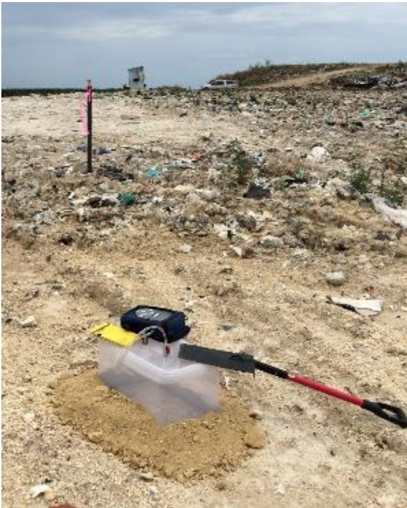
Figure 3.6: Gas and Emissions Monitoring at George Town Landfill
