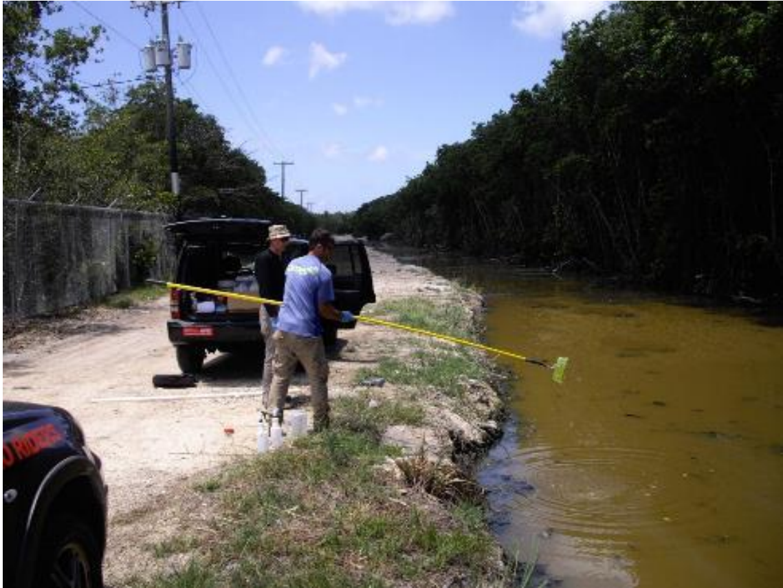
Figure 3.5: The Collection of Surface Water Samples from the Dyke to the North of George Town landfill
